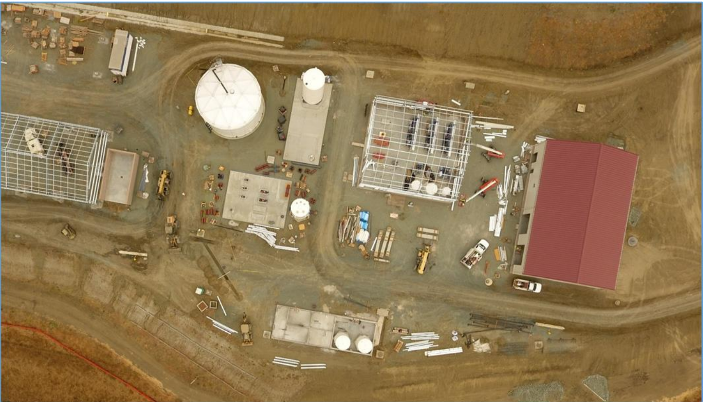
June 30, 2021 – (L to R): Vehicle Equipment Storage Canopy, Wash Rack, Product Water Tank, IPR/Outfall Pump Station, Chem Facility (lower frame), Calcite Contactor, RO/UV Bldg, and Maint Bldg.
