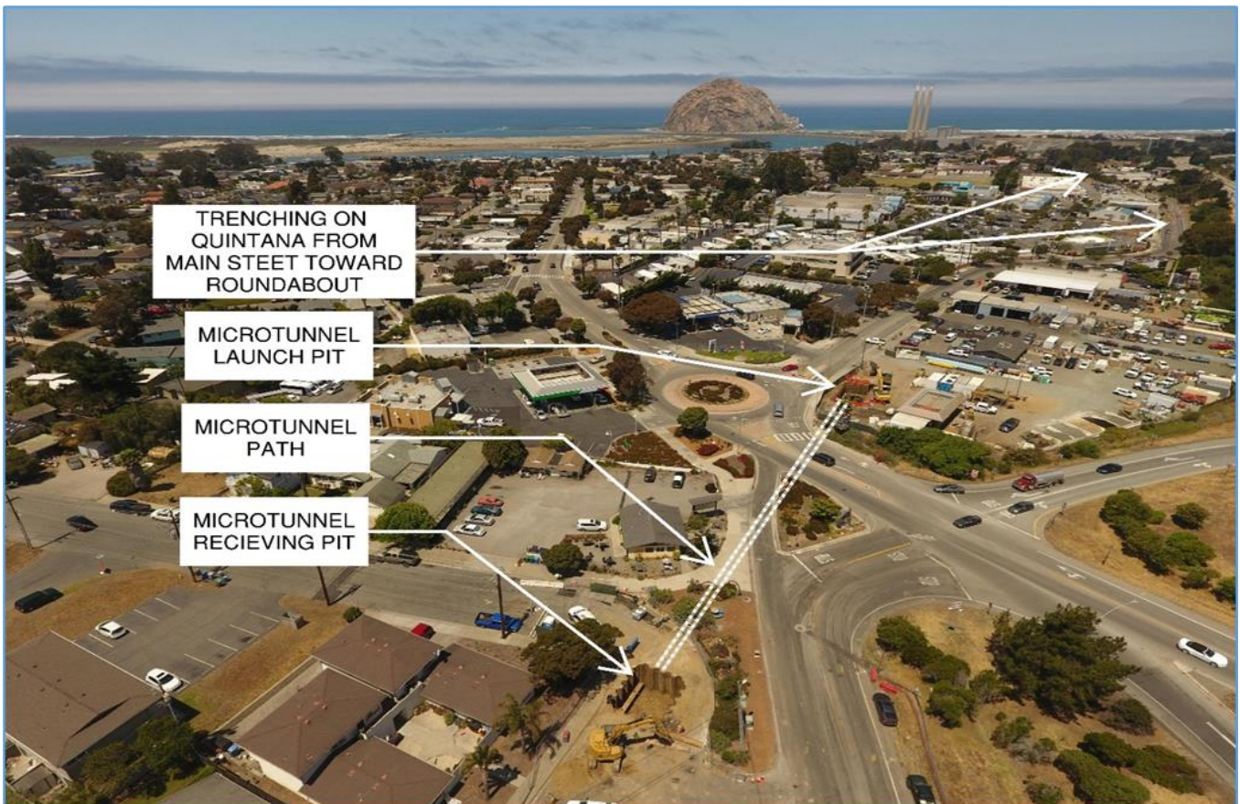
June 30, 2021 – Morro Bay Blvd Roundabout Microtunnel (note launch pit, receiving pit and Microtunnel path)
