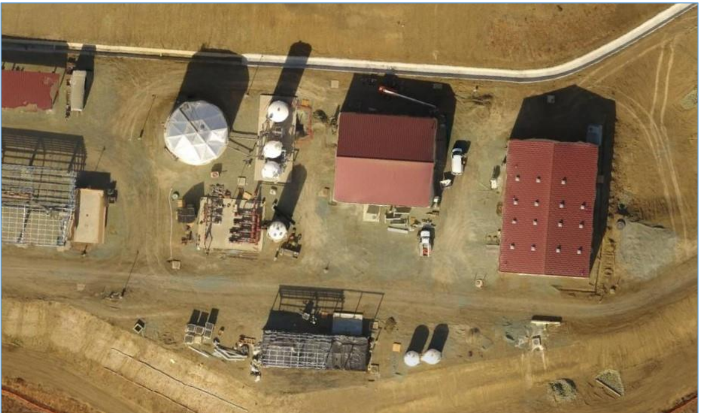
Sept. 30, 2021 – (L to R): Vehicle Equipment Storage Canopy, Wash Rack, Product Water Tank, IPR/Outfall Pump Station, Chem Facility (lower frame), Calcite Contactor, RO/UV Bldg, and Maint Bldg.
