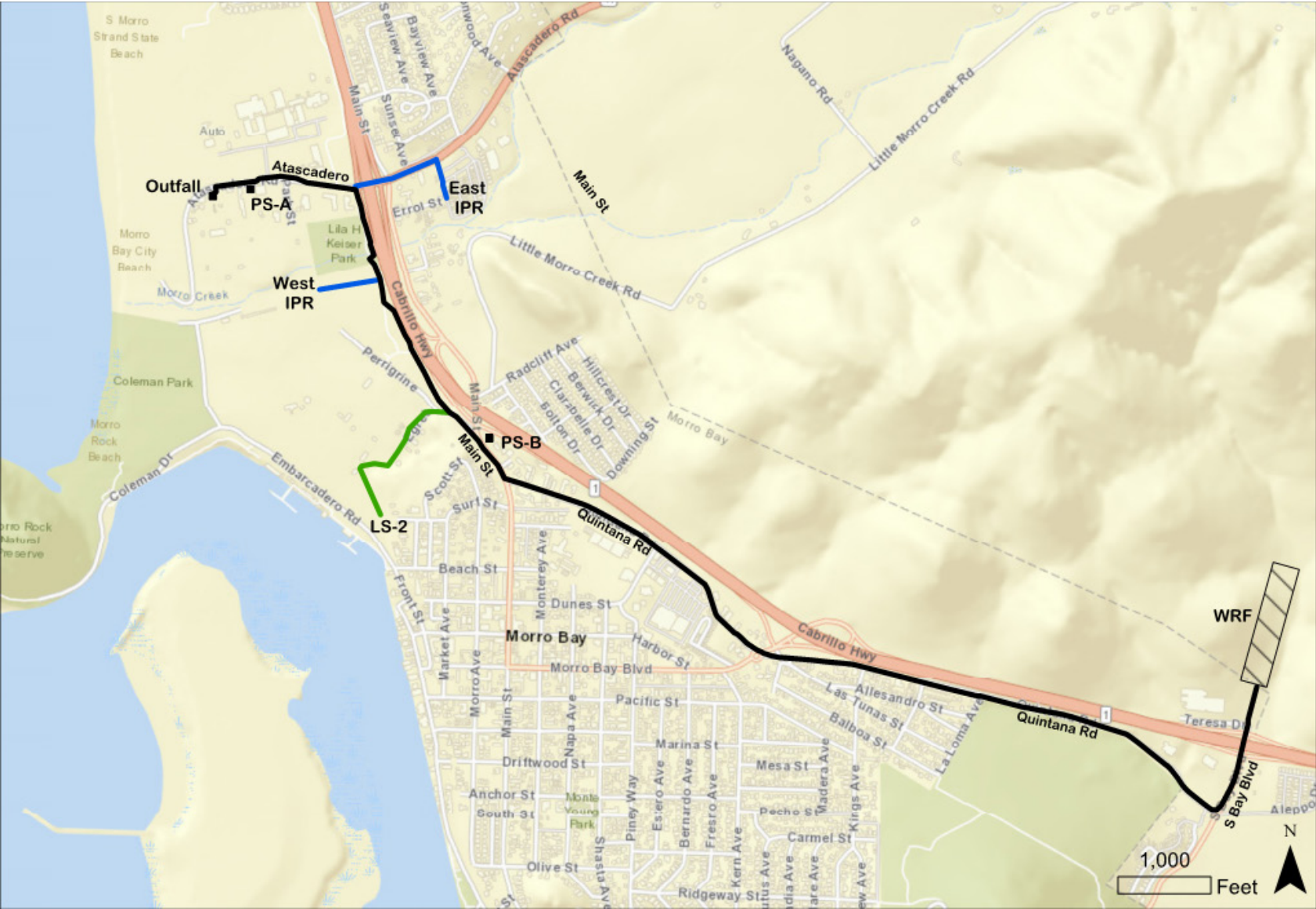
Figure 4 Conveyance Facilities Pipeline Alignment
