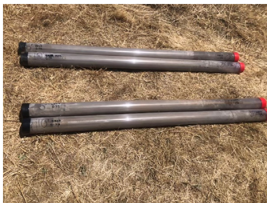
Pipeline Alignment Cores (Shallow Cores)
