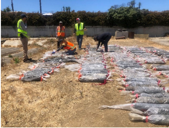
Well Site Cores (Deep Sonic Cores)
