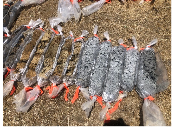
Well Site Cores (Deep Sonic Cores)
