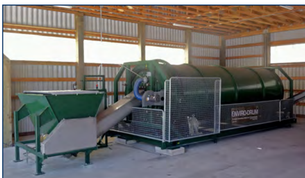
Figure 5-5 In-Vessel Composting System (DTEnvironmental)
