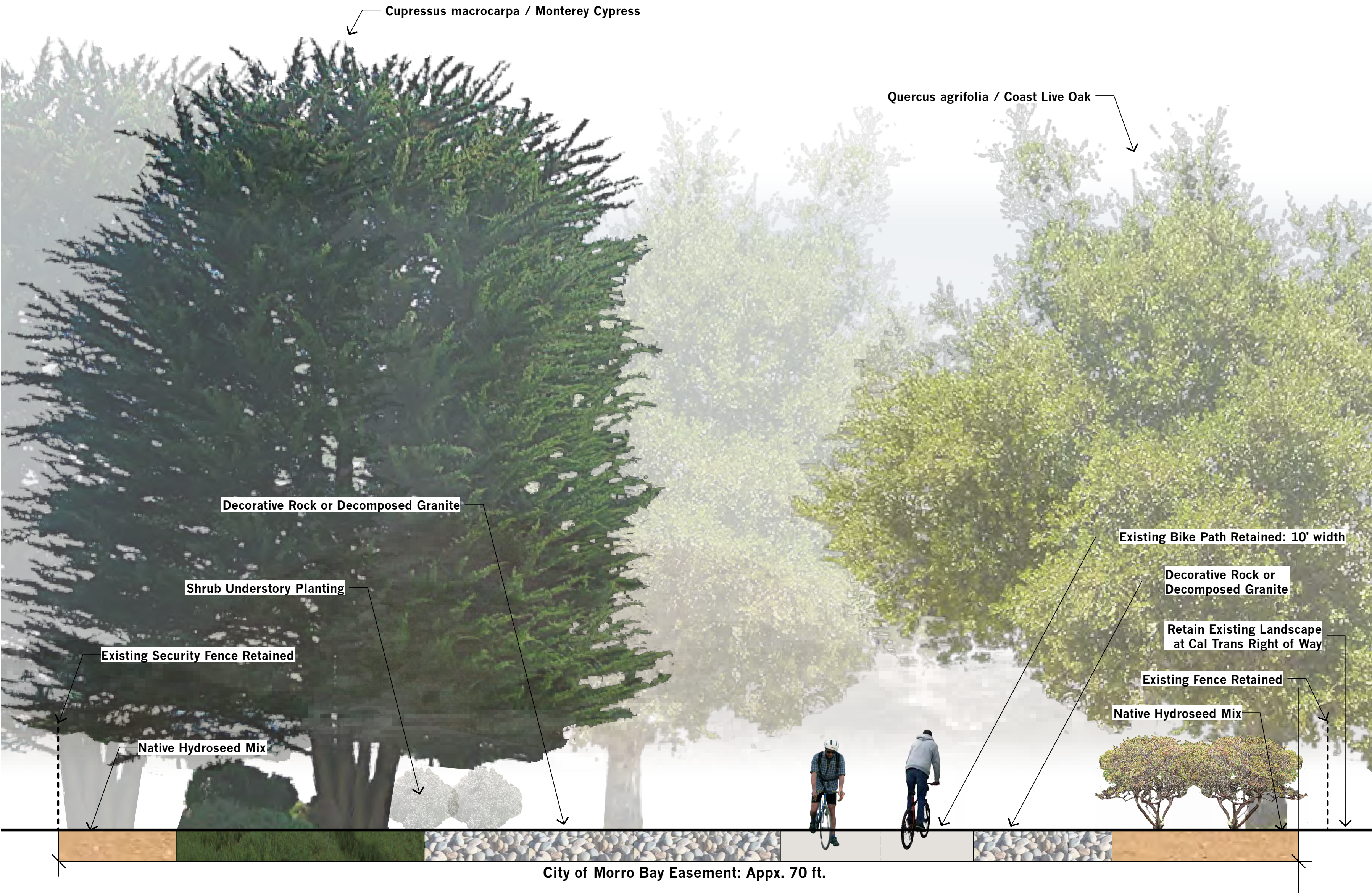
Typical Cross Section- Revegetation Plan - Scale: 1/4" = 1'-0"
