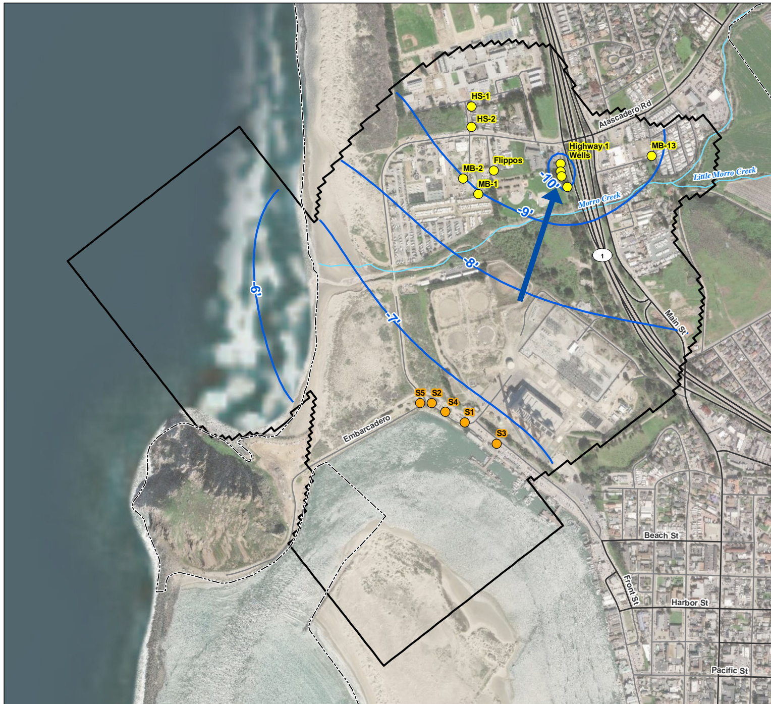
FIGURE 4 Morro Bay Full Pumpage Final Groundwater Elevations Morro Bay Water Reclamation Facility Morro Bay, CA
