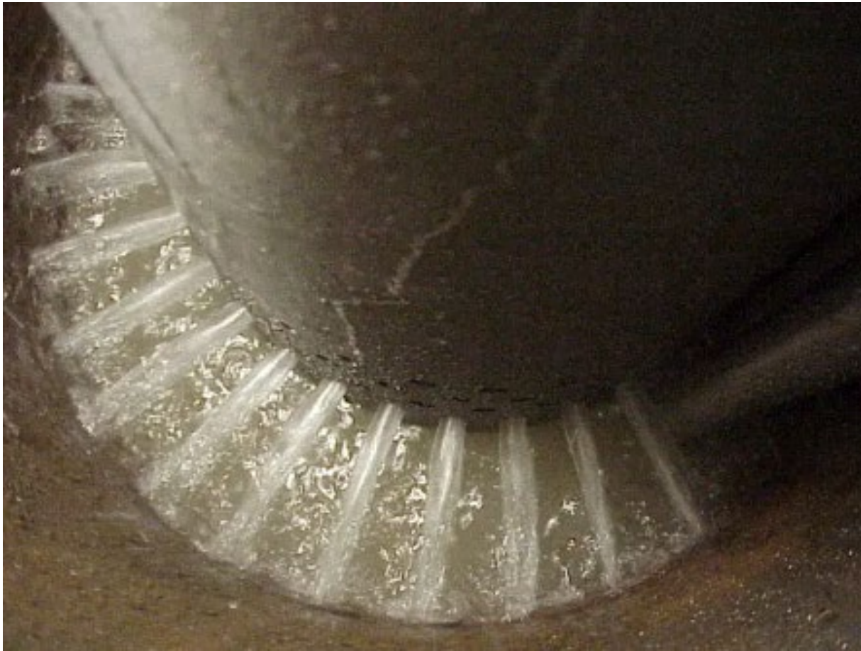
Figure 6-6 3R Valve Orifices and Injection Flow Pattern
