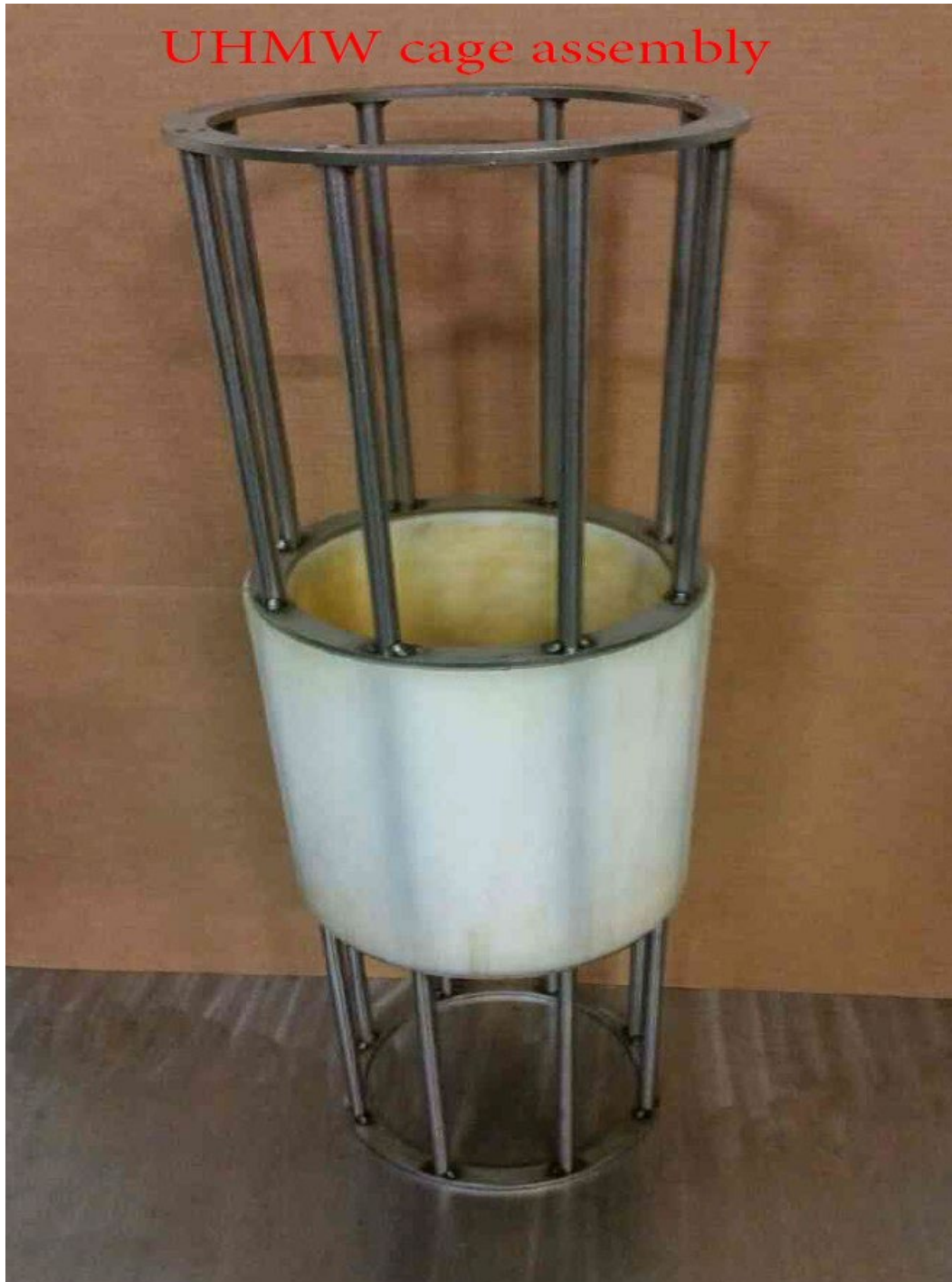
Figure 6-5 3R Valve Cage Assembly with UHMW Sleeve
