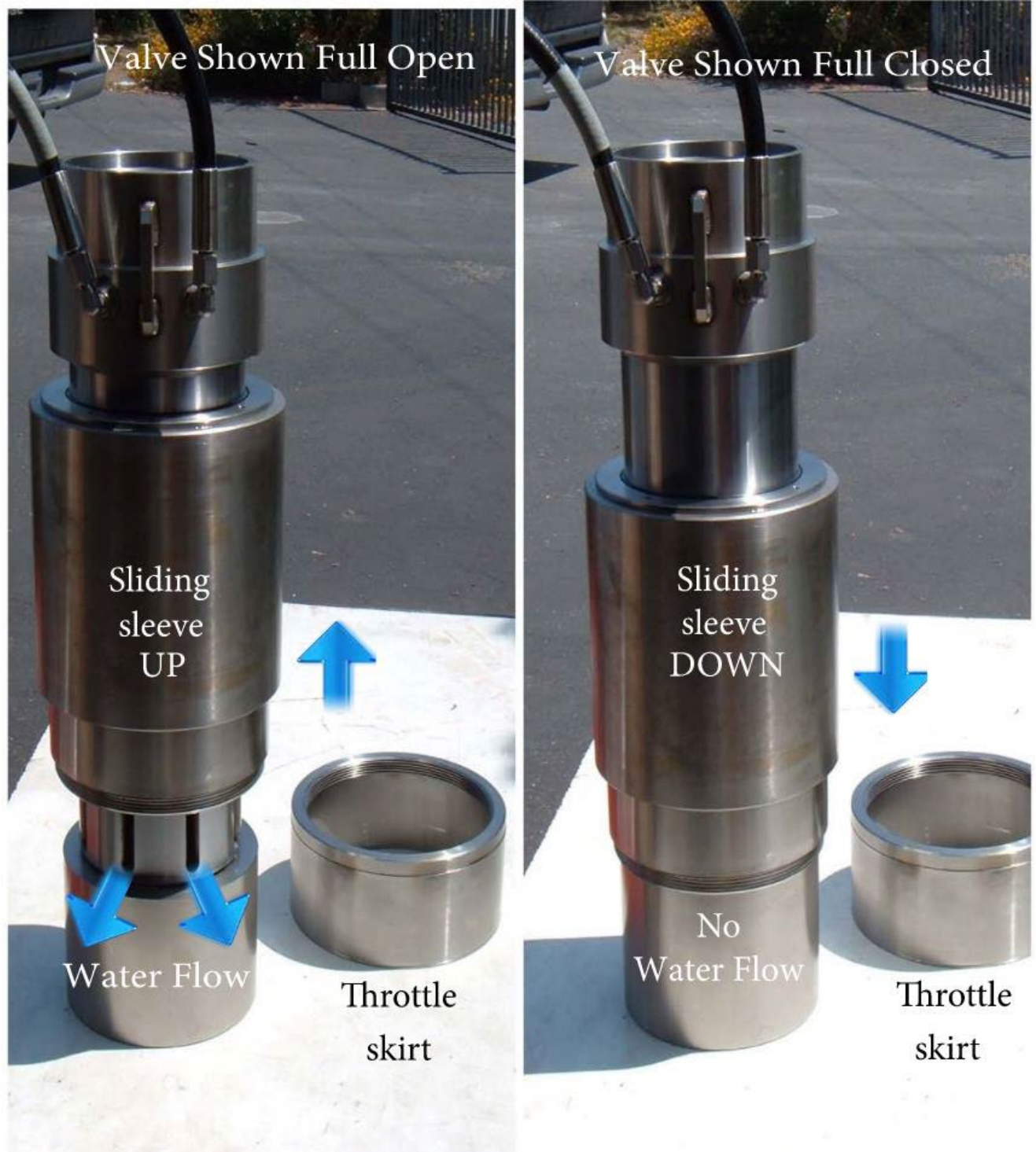
Figure 6-9 V-Smart Valve Positions
