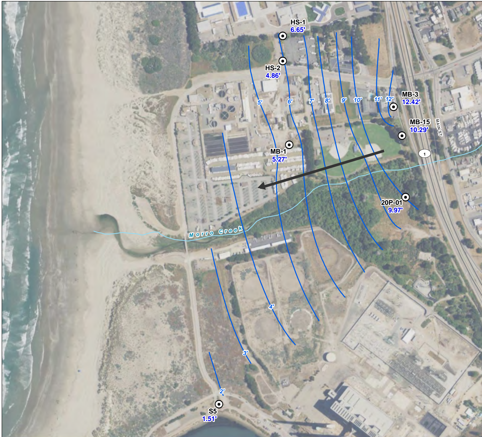
FIGURE 3 July 2021 Groundwater Elevation Contours Morro Bay IPR Program Interim Tracer Test Workplan
