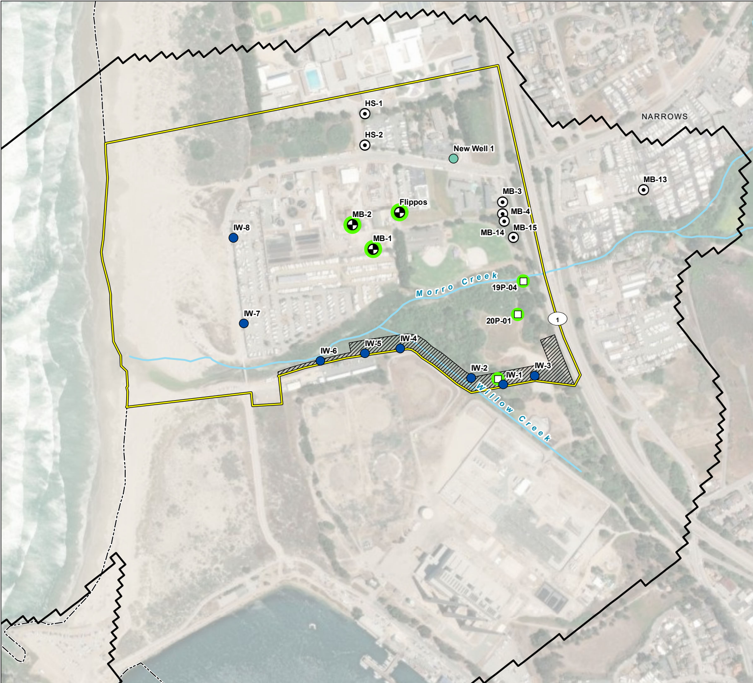
FIGURE 31 Recommended Injection Well Locations Morro Bay IPR Project Basis of Design Report
